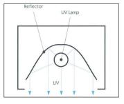
UV irradiation with a parabolic reflector
