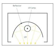
UV irradiation with an elliptical reflector
